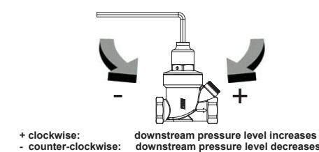
+ clockwise: downstream pressure level increases
